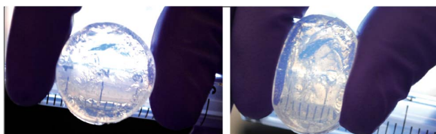
Fig. 6 Digital photographs of a PMMA-MAA-EGD DX microgel before and after compression.
