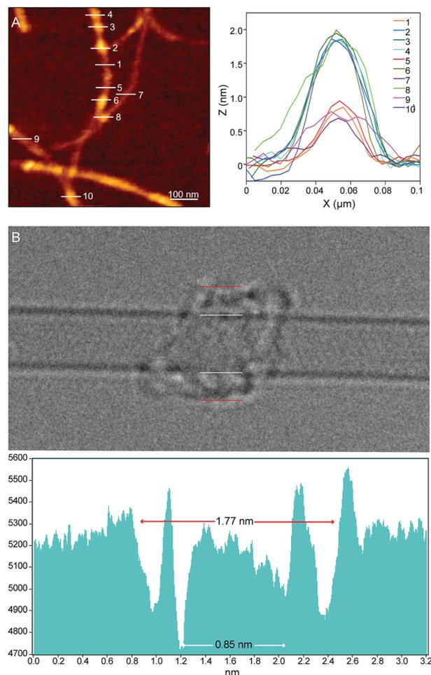
**Fig. 2** (A) AFM topographic image of a suspension of **MINT-por** in TCE and corresponding height profiles along the lines marked in the topographic image. (B) AC-HRTEM image of an individual SWCNT functionalized by a single macrocycle in **MINT-por** and corresponding profiles (white lines and arrows mark SWCNT diameter, red lines and arrows mark **mac-por** diameter).
