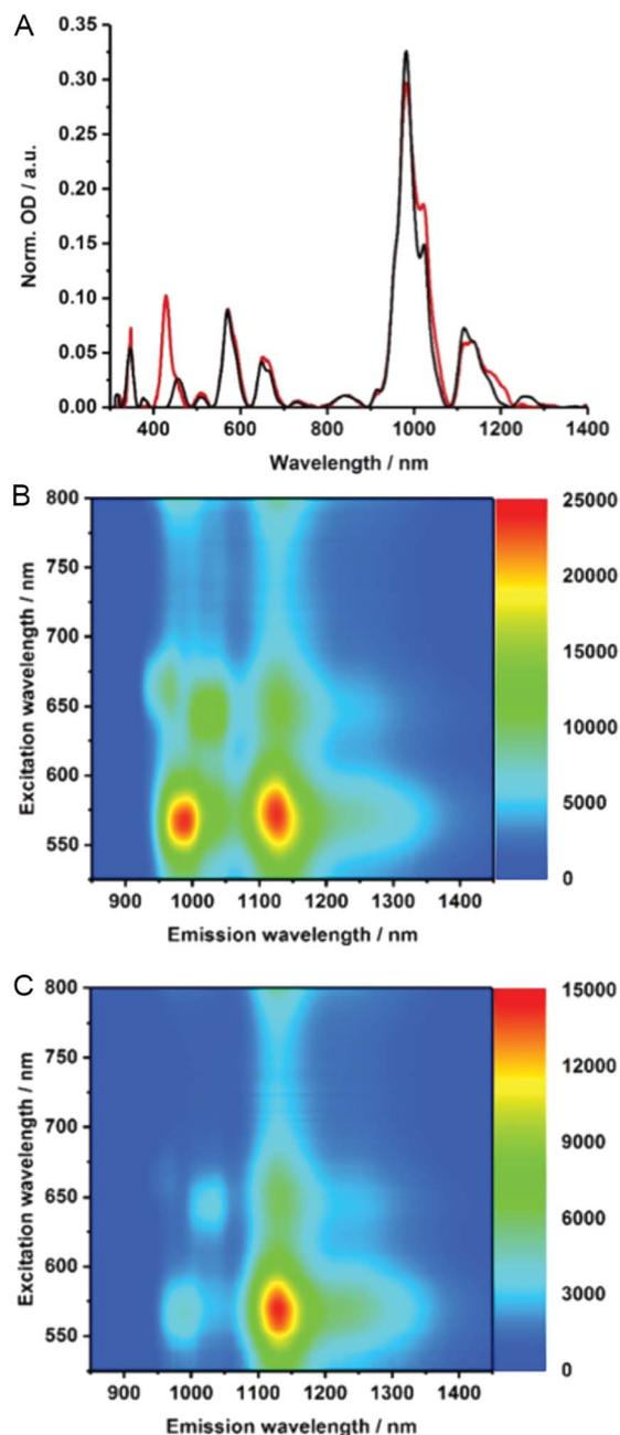
Fig. 3 (A) Normalized absorption spectra of (6,5)-enriched SWCNTs (black), and **MINT-por** (red) in D<sub>2</sub>O/SDBS (1 wt%, rt), baseline-corrected and normalized to the (7,6)-SWCNT absorption at 1136 nm. 3D nIR fluorescence spectra of (B) (6,5)-enriched SWCNTs and (C) **MINT-por** in D<sub>2</sub>O/SDBS (1 wt%, rt) with OD of 0.21 at 570 nm.
