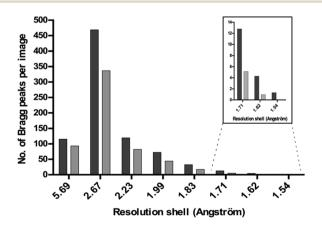
Fig. 6 The diffraction quality (measured as the number of Bragg peaks per image) as a function of the resolution of native (light grey) and Tb—Xo4 (dark gray) HEWL crystals obtained under shared crystallization conditions.
