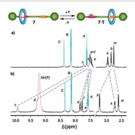
Fig. 4 Selected regions of the <sup>1</sup>H NMR spectra (400 MHz, CD<sub>2</sub>Cl<sub>2</sub>, 298 K) of (a) shuttle 7 and (b) after adding an excess (20 equiv.) of *N*-hexylthymine (T) (see Scheme 2 for signal assignments).
