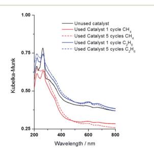
Fig. 9 DR UV-vis spectra of 1.1 wt% Fe/ZSM-5\_#4 employed in the oxidation of methane and ethane measured after one (1) and five (5) reaction cycles using H<sub>2</sub>O<sub>2</sub> as oxidant. Test conditions as in Fig. 8, catalysts analysed at room temperature after air drying overnight.
