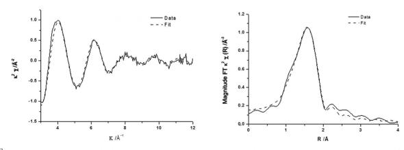
Fig. 7  $k^2$  experimental  $\chi$  data and fit (left) along with associated Fourier transform (right) for calcined 0.4 wt% Fe-0.4 wt% Cu/ZSM-5\_#13 prepared by CVI.
