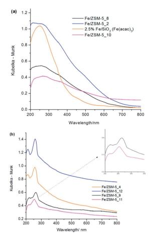
Fig. 2 DR UV-vis absorbance spectra of various Fe/ZSM-5 and Fe/SiO $_2$  catalyst materials (a) heat treated at 550 °C in air for 3 h and (b) catalysts heat treated at 550 °C in 5% H $_2$ /Ar for 3 h.
