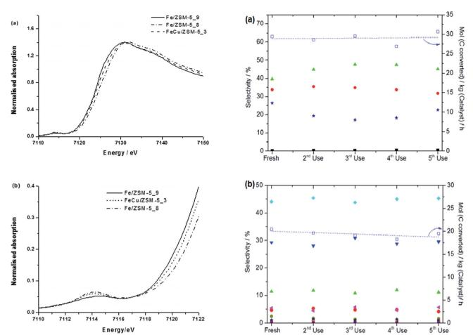
Fig. 6 (a) XANES spectra and (b) expanded pre-edge region of XANES spectra of 0.4 wt% Fe-0.4 wt% Cu/ZSM-5\_#13 CVI samples.
