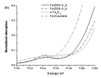
Fig. 4 (a) XANES spectra and (b) expanded pre-edge region from various 0.4 wt% Fe/ZSM-5(30) CVI samples.
