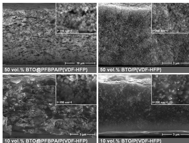
Fig. 7 Cross-section SEM images of spin-coated phosphonic acid modified BTO@PFBPA/P(VDF-HFP) (left) and pure BTO/P(VDF-HFP) composites films (right) with different BaTiO<sub>3</sub> volume fractions.
