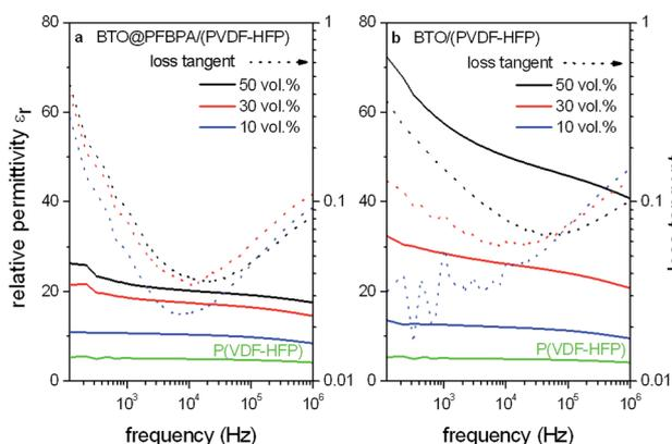
Fig. 9 Relative permittivities and loss tangents of spin-coated phosphonic acid modified BTO@PFBPA/P(VDF-HFP) (a) and pure BTO/P(VDF-HFP) (b) composite films with different BaTiO<sub>3</sub> volume fractions compared to the pure polymer.
