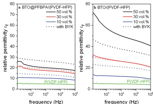
Fig. 10 Relative permittivities of composite films from phosphonic acid modified BTO@PFBPA/P(VDF-HFP) (a) and pure BTO/P(VDF-HFP) (b) containing different BaTiO<sub>3</sub> volume fractions with and without addition of the dispersant BYK-W 9010.
