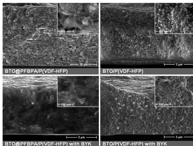
Fig. 8 Cross-section SEM images of composite films from phosphonic acid modified BTO@PFBPA/P(VDF-HFP) (left) and pure BTO/P(VDF-HFP) (right) with and without addition of the BYK dispersant. The BTO content was 30 vol% in all cases.
