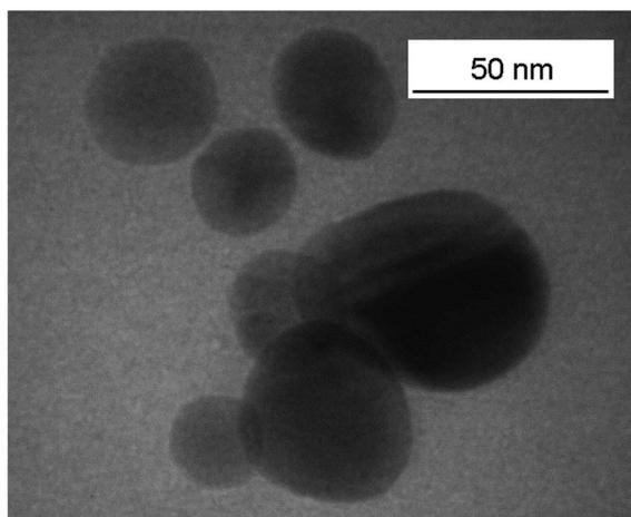
Fig. 1 TEM bright-field image of BaTiO<sub>3</sub> particles synthesized by the sol-gel procedure.
