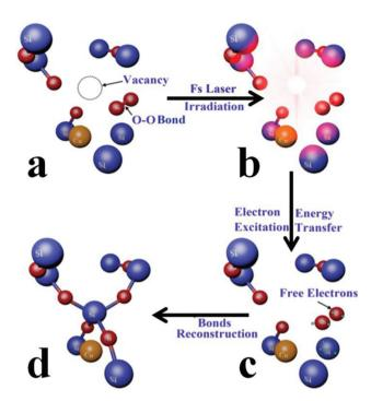
Fig. 6 Repair process. The schematic diagram of the nanoscale defects repair process in four stages, as (a) defects in fused silica implanted by the focused Cu ion beam, (b) precisely controlled femtosecond laser irradiation with a laser fluence approximately 0.2 J cm<sup>-2</sup>, (c) energy transition from the electromagnetic field to electrons, and (d) bond reconstruction.
