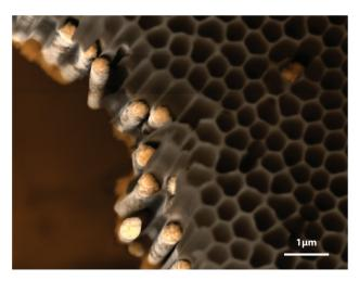
**Fig. 5** Scanning electron micrograph of Pt nanowires grown in an anodic alumina template (10 mM H<sub>2</sub>PtCl<sub>6</sub>, pH 1.5, –250 mV vs. Ag/AgCl, 30 minutes).
