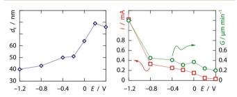
Fig. 1 Effect of the applied potential E (vs. Ag/AgCl) on the wall thickness  $d_{\rm t}$  of the nanotubes (after 3.5 minutes of growth), the total galvanic current i (exposed macroscopic electrode area 0.05 cm²) and the nanotube growth rate G (6 mM PtCl<sub>4</sub>²-, 1 M H<sub>2</sub>SO<sub>4</sub>). The uncertainty on  $d_{\rm t}$  is estimated at  $\pm 20$  nm.
