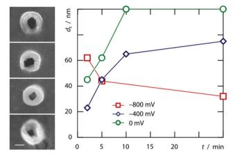
Fig. 4 Variation of the tube morphology with deposition time. Left, scanning electron micrographs of Pt nanotubes taken axially after 2, 5, 10, and 30 minutes of growth (2 mM  $\rm H_2PtCl_6$ , pH 3.8,  $\rm -400$  mV); scale bar: 100 nm. Right, graphical representation of the data gathered at  $\rm -800$ ,  $\rm -400$ , and 0 mV (vs. Ag/AgCl). The uncertainty on  $\rm d_t$  is estimated at  $\rm \pm 20$  nm.
