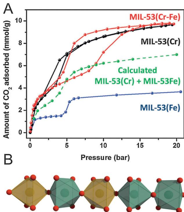
Fig. 20 (A) Comparison of the CO<sub>2</sub> adsorption isotherms of MIL-53(Fe–Cr), MIL-53(Fe), and MIL-53(Cr). (B) One dimensional SBU chains in MIL-53(Fe–Cr). Green and orange polyhedra represent iron and chromium SBUs, respectively. Red spheres represent oxygen atoms. (Reprinted with permission.<sup>151</sup> Copyright 2012. The Royal Society of Chemistry.)
