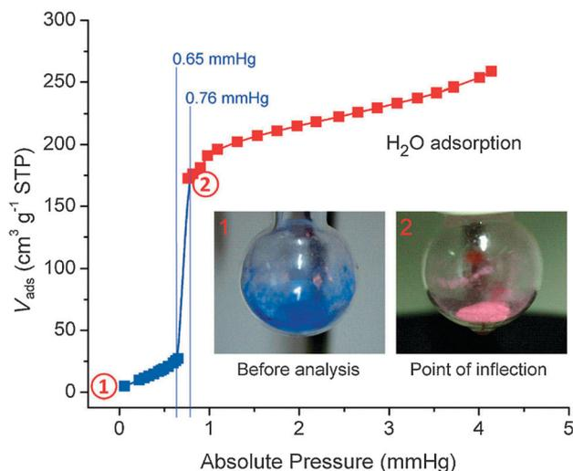
Fig. 33 Color change of [Co<sub>1.5</sub>(tipb)(SO<sub>4</sub>)(bdc)<sub>0.5</sub>]<sub>n</sub> during H<sub>2</sub>O adsorption. (Reprinted with permission.<sup>228</sup> Copyright 2012 John Wiley and Sons.)
