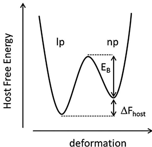
Fig. 29 Schematic of the host free energy landscape for the "dry" bistable framework.
