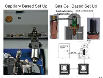
Fig. 24 Capillary based experimental setup (left) (Reprinted with permission 161) and gas cell, based on closed cycle He-cryostat (right) (Reprinted with permission. 162 Copyright 2014. Elsevier.)
