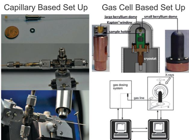
Fig. 24 Capillary based experimental setup (left) (Reprinted with permission<sup>161</sup>) and gas cell, based on closed cycle He-cryostat (right) (Reprinted with permission.<sup>162</sup> Copyright 2014. Elsevier.)
