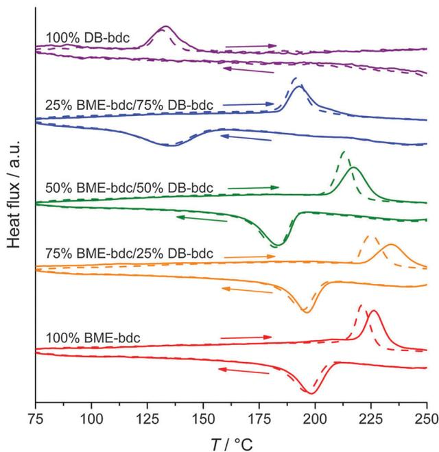
Fig. 21 DSC curves of  $[\text{Zn}_2(\text{BME-bdc})_{2x}(\text{DB-bdc})_{2-2x}\text{dabco}]_n$  solid solutions. (Reprinted with permission.<sup>57</sup> Copyright 2013 John Wiley and Sons) and Sons.
