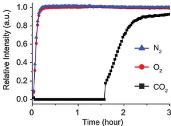
Fig. 31 Breakthrough curve for CID-3 for mixture  $\text{CO}_2 : \text{O}_2 : \text{N}_2 = 1 : 21 : 78$  at total pressure of 0.5 MPa. (Reproduced with permission.<sup>223</sup> The Royal Society of Chemistry.)
