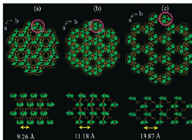
**Fig. 10** Simulated crystal structures of the MIL-88A framework in its np (a), as (b), and lp (c) forms. (Reprinted with permission.<sup>87</sup> Copyright 2005 American Chemical Society.)
