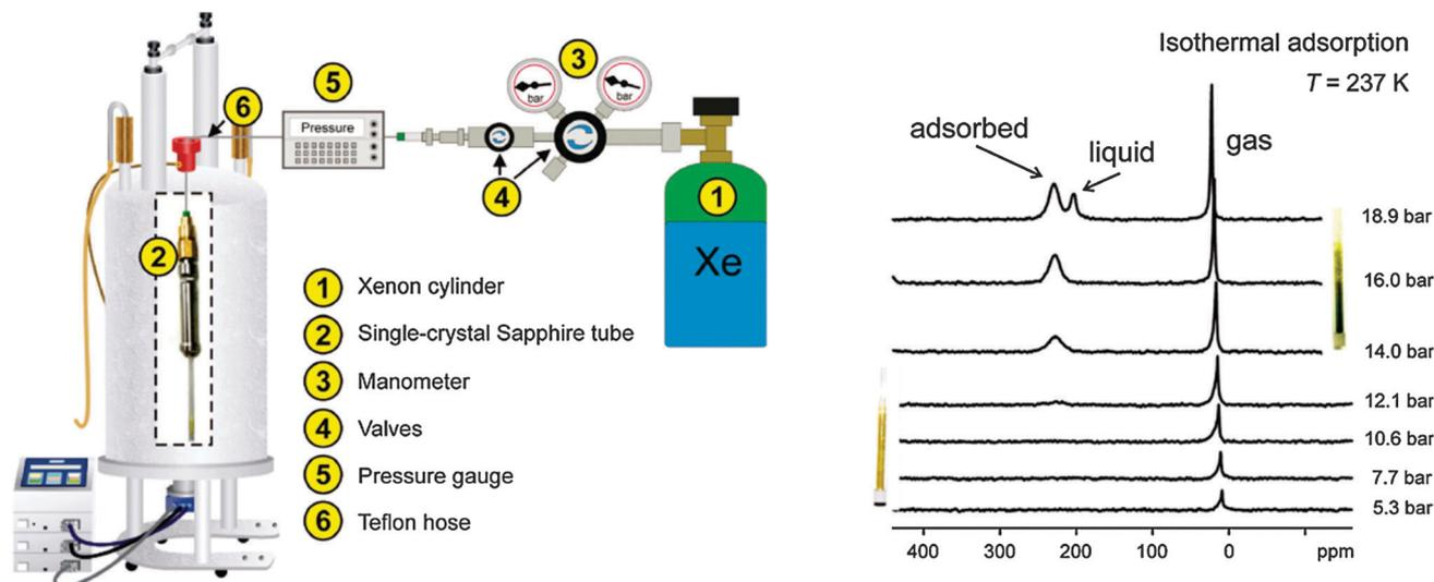
Fig. 25 Schematic representation of an apparatus for high pressure *in situ*  $^{129}\text{Xe}$  NMR experiments under variable thermodynamic conditions (left). *In situ*  $^{129}\text{Xe}$  NMR spectra recorded during the adsorption and desorption of Xenon on DUT-8(Ni) at 237 K (right). (Reprinted with permission<sup>180</sup> Copyright 2011. American Chemical Society.)
