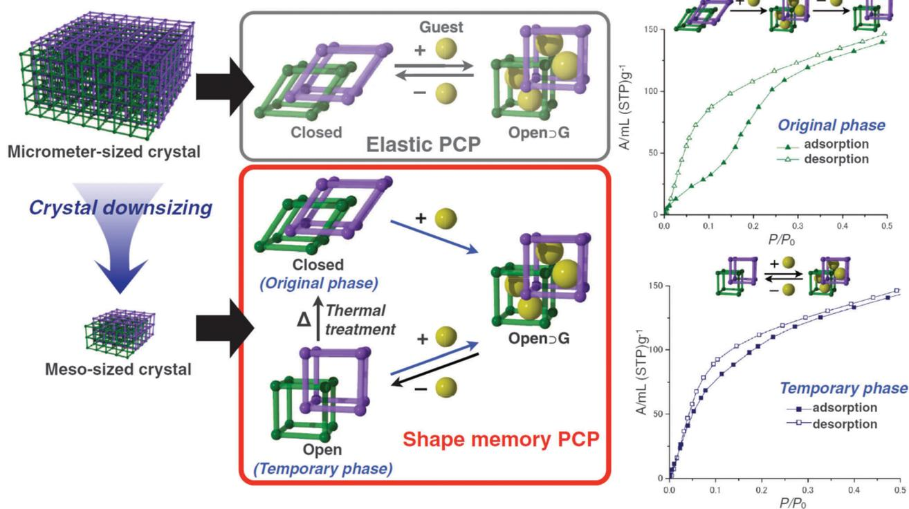
Fig. 7 Schematic depiction of the flexible behaviour of micro-sized [Cu<sub>2</sub>(bdc)<sub>2</sub>(bipy)]<sub>n</sub> in comparison with meso-sized [Cu<sub>2</sub>(bdc)<sub>2</sub>(bipy)]<sub>n</sub>. Right – methanol adsorption isotherms of the closed (original phase) and the open (temporary phase) of meso-sized [Cu<sub>2</sub>(bdc)<sub>2</sub>(bipy)]<sub>n</sub>. (Reprinted with permission.<sup>76</sup> Copyright 2013. American Association for the Advancement of Science.)
