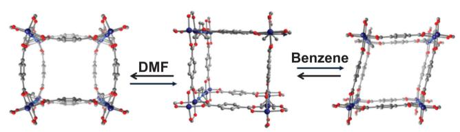
Fig. 12 Crystal structure of  $[Zn_2(bdc)_2(dabco)]_n$  (view along c direction): left – as synthesized phase; middle – activated phase; right – after infiltration of benzene. Colour code: Zn - blue, O - red, C - grey. H atoms are omitted for clarity.
