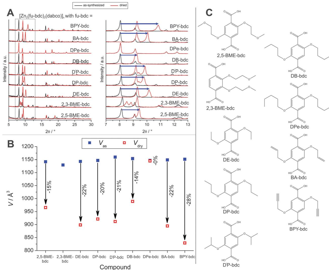
Fig. 17 (A) Powder patterns of as-synthesized (black) and dried (red)  $[\text{Zn}_2(\text{fu-bdc})_2(\text{dabco})]_n$ . (B) Evolution of the cell parameters during the transitions from the as-synthesized **lp** to the dried **np** of the framework. (C) Listing of the linkers that were used to prepare the discussed pillared-layered frameworks. (Reprinted with permission.<sup>138</sup> Copyright 2012. American Chemical Society.)
