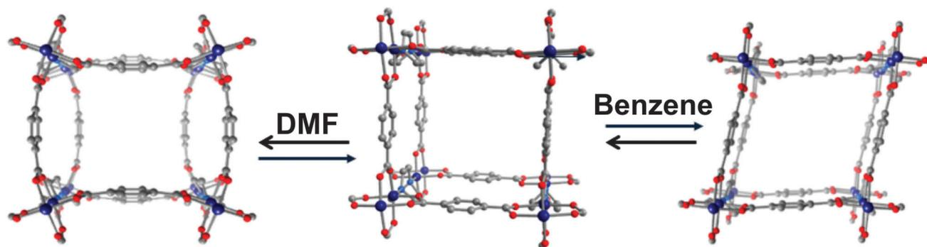
Fig. 12 Crystal structure of  $[\text{Zn}_2(\text{bdc})_2(\text{dabco})]_n$  (view along *c* direction): left – as synthesized phase; middle – activated phase; right – after infiltration of benzene. Colour code: Zn – blue, O – red, C – grey. H atoms are omitted for clarity.
