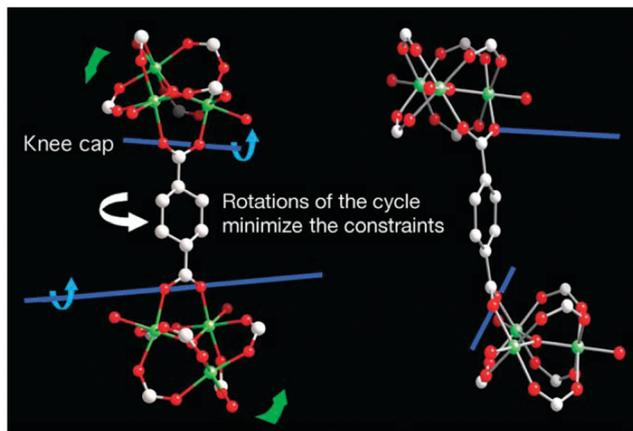
Fig. 11 Depiction of the hinge in MIL-88 around which the rotation that induces the pore swelling occurs. (Reprinted with permission.<sup>133</sup> Copyright 2007 American Association for the Advancement of Science.)
