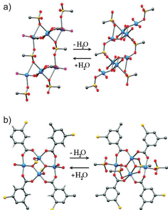
Fig. 23 Structural transformations in Cu-SIP-3 during hydration/dehydration: (a) Chains of the copper tetramers in the low-temperature (left) and high-temperature (right) structures. (b) Copper tetramers in the low-temperature (left) and high-temperature (right) structures. Color codes: Blue balls – copper atoms; red balls – oxygen atoms; yellow balls – sulfur atoms; grey balls – carbon atoms (Reprinted with permission from,<sup>155</sup> Copyright 2010. American Chemical Society.)
