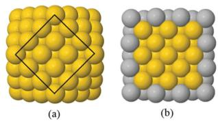
Fig. 1 Examples of the cuboctahedral structure: (a) Au<sub>147</sub>; and (b) a cross section of Au<sub>55</sub>@Ag<sub>92</sub> core@shell structure. Yellow and grey spheres represent Au and Ag, respectively. For clarity, the (100) surface in (a) has been highlighted with a black line.
