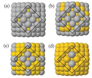
Fig. 4 Minimum energy alloy structures of cuboctahedral as calculated using atomic-swap basin-hopping with the Gupta potentials: (a) Au<sub>13</sub>Ag<sub>134</sub>, (b)  $Au_{55}Ag_{92}$ , (c)  $Au_{92}Ag_{55}$  and (d)  $Au_{134}Ag_{13}$ . Yellow spheres represent Au, grey spheres Ag.
