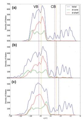
Fig. 9 Density of states (DOS) profiles for (a)  $Ag_{147}$ , (b)  $Au_{147}$  and (c)  $Au_{74}Aq_{73}$ . A key is provided.  $E_{\rm F}$  is given as a black dotted line, with the valence band maximum (VBM) and conduction band minimum (CBM) in purple and orange for anatase and rutile TiO2, respectively. 77 A Gaussian broadening of 0.05 eV has been used on the electronic states
