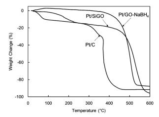
Fig. 8 TGA of Pt/SiGO, Pt/C, and Pt/GO-NaBH<sub>4</sub> under air. Heating rate: 2 °C min<sup>-1</sup>.
