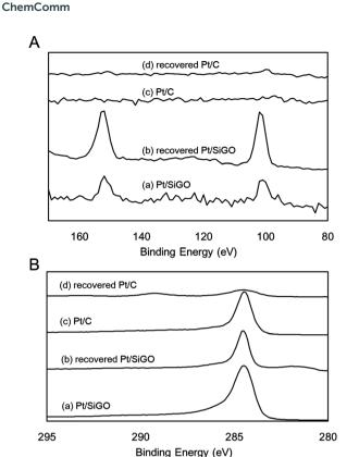
Fig. 5 XPS of (A) Si 2p and 2s, and (B) the C 1s regions of Pt/SiGO and Pt/C before and after the methane oxidation reaction.
