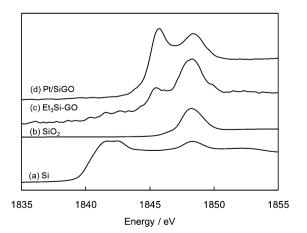
Fig. 6 Si K-edge XANES spectra of (a) Si(0), (b) SiO<sub>2</sub>, (c) Et<sub>3</sub>Si-modified GO, and (d) Pt/SiGO
