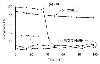
Fig. 3 Time course of the catalytic activity of methane conversion under oxygen at 400 °C. (a) Pt/C, (b) Pt/SiGO, (c) Pt/GO-EG, and (d) Pt/GO-NaBH<sub>4</sub>
