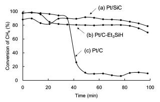
Fig. 9 Catalytic activities of the hydrosilane-treated catalysts.
