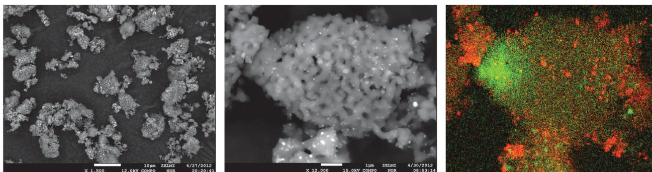
Fig. 4 SEM images of fresh Cat-2 ( $Mn_xO_y-Na_2WO_4/SiO_2$ ) and EDX-mapping of W L-edge (green) and Mn K-edge (red).
