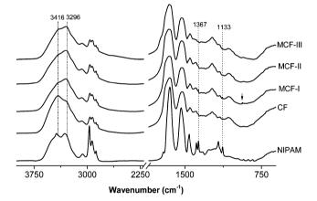
**Fig. 2** FTIR spectra of CF, MCF-I, MCF-II and MCF-III. For CF, MCF-I, MCF-II and MCF-III, the intensities are normalized at  $3200 \text{ cm}^{-1}$ . The spectra are offset, and curves are shifted vertically for clarity.
