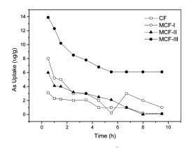
**Fig. 8** The As(III) sorption kinetics of 0.1 g L<sup>-1</sup> of CF, MCF-I, MCF-II, MCF-III for concentrations of 200  $\mu$ g L<sup>-1</sup> of sodium arsenite solution at 20 °C.
