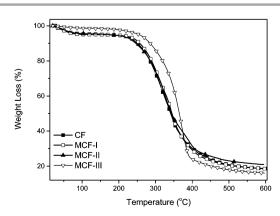
Fig. 6 TGA curves of CF, MCF-I, MCF-II, and MCF-III.
