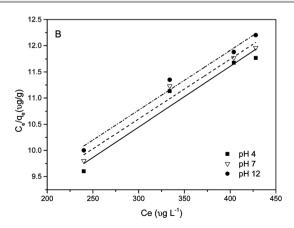
Fig. 10 Linearized (A) Freundlich and (B) Langmuir isotherms for the arsenic adsorption on MCF-III at different pH at 20 °C.
