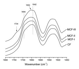
**Fig. 3** FTIR spectra of the amide I region for CF, MCF-II, MCF-II and MCF-III. For easier comparison, intensities are normalized in all spectra at 1640 cm<sup>-1</sup>. The spectra are offset, and curves are shifted vertically for clarity.
