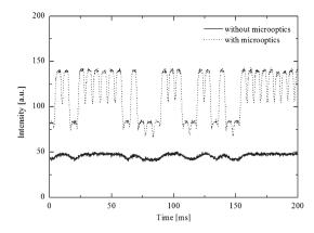
**Fig. 4** Measured fluorescent signals resulting from the microoptics integrated system as compared to a conventional device, using droplets containing 100 μM (big peaks) and 50 μM (small peaks) fluorescein.
