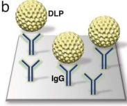
Fig. 1 Schematic of a microfluidic chamber (a) that accommodates biological assemblies (yellow) in solution while inside a TEM column. (b) Magnified view of the chamber surface decorated with IgG antibodies (blue) against the DLP outer capsid protein, VP6
