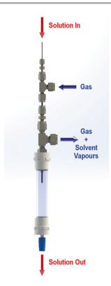
Fig. 1 Graphical representation of the device used for the solvent evaporation/ switch (see also ESI+).
