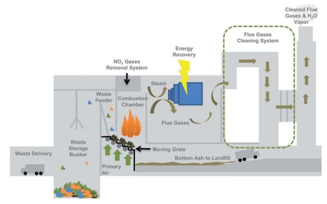
Fig. 1 Schematic of grate incinerator operation.<sup>56</sup>
