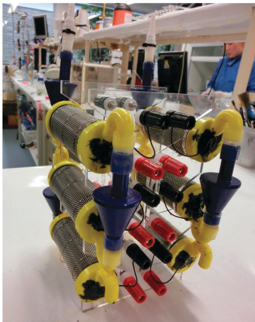
Fig. 1 Two cascades of 3 MFCs each, assembled with air-gap adaptors.
