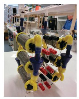
Fig. 1 Two cascades of 3 MFCs each, assembled with air-gap adaptors.
