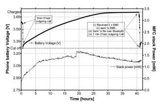
**Fig. 4** MFC stack power behaviour during the charging and operation of the Samsung GT-E2121B mobile phone. During the operation, 2 outgoing calls were made, 2 text messages were received and 1 was sent, and Bluetooth® was enabled for synchronising with another handset for file transfer.
