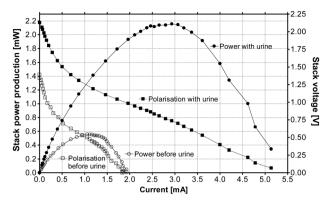
**Fig. 3** Power and polarisation curves from the ceramic 12× MFC stack, when fed with acetate–tryptone extract (open symbols) and urine (closed symbols).
