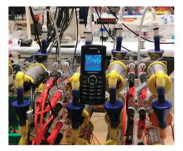
Fig. 5 Samsung GT-E2121B powered by the ceramic MFC stack
