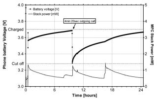
Fig. 6 MFC stack (24 × 6.25 mL units) powering the Samsung mobile phone, when fed with neat urine
