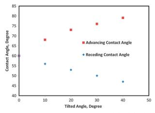
**Fig. 7** Advancing and receding contact angles *versus* titled angle for a bubble submerged in liquid.
