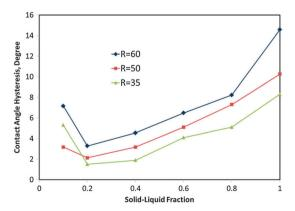
**Fig. 3** Contact angle hysteresis *versus* solid–liquid fraction for a droplet on the tilted surface; for three different drop diameters (*R*).
