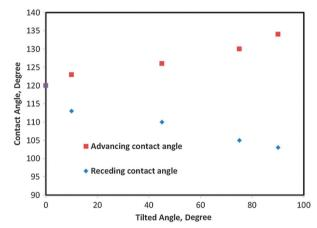
Fig. 6 Advancing and receding contact angles versus titled angle for a droplet on the tilted surface.
