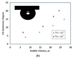
**Fig. 9** CA hysteresis obtained by experiment for (a) droplets of different sizes on concrete TiO<sub>2</sub> coated tiles, and (b) bubbles of different sizes on the AI sample, for different tilt angles (TA).
