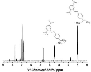
Fig. 1  $\,^{-1}$ H-NMR patterns of MR-MIL-125(Ti) digested in KOH. The alkyl signals confirm the designed modification.
