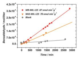
Fig. 3 Photocatalytic benzaldehyde evolution. No catalyst (grey), NH<sub>2</sub>-MIL-125(Ti) (orange) and MR-MIL-125(Ti) (red). 200 µL of benzyl alcohol/12 mL CH<sub>3</sub>CN, 150 W Xe lamp. 12 mg of NH<sub>2</sub>-MIL-125(Ti) and 18 mg of MR-MIL-125(Ti).
