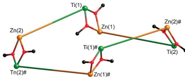
**Fig. 5** A view of the complex  $[Ti_4Zn_4L_8(\mu-OMe)_8]$  showing only the eight metal ions and the bridging methoxide ligands which connect each Ti/Zn double helicate (a long 'edge' in this view) into a cyclic tetramer (C = black, O = red). Atoms labeled '# are at equivalent position  $(-x, y, 0.5 - z)$ .
