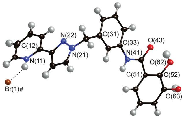
**Fig. 1** Molecular structure of  $H_2L \cdot HBr$ . Non-H atoms are shown with 40% thermal ellipsoids, the hydrogen-bond between the protonated pyridine and the bromide anion is shown with a dotted line. Atoms labeled '#' are at equivalent position  $(-x, 1 - y, z)$ .
