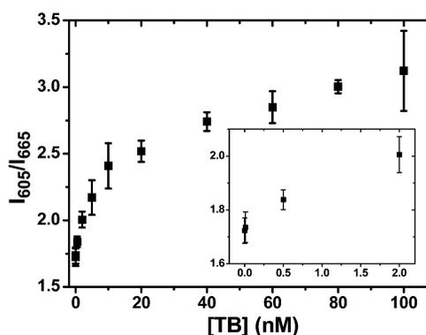
**Fig. 4** Label-free detection of thrombin using the CFCC clicked QD-DNA aptamer sensor using 2 nM QD-TBA<sub>20</sub> pre-hybridized with DNA12-SM (60 nM) in PBS containing 20  $\mu$ M BSA. A typical calibration curve showing the  $I_{605}/I_{665}$  ratio as a function of thrombin concentration [TB] (inset: the response over 0–2 nM of [TB]).
