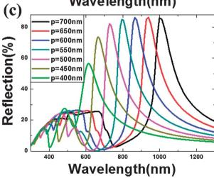
**Fig. 2** (a) SEM image showing the top view of a silver nanorod array with period p=550 nm. (b) Measured and (c) calculated reflection spectra for nanorod arrays with periodicities from 400 nm to 700 nm. The arrow indicates increasing periodicities.
