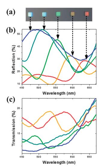
**Fig. 5** (a) Optical image showing the reflective colors from different silver nanorod arrays. Measured reflection (b) and transmission (c) spectra of the corresponding arrays as a function of wavelengths.
