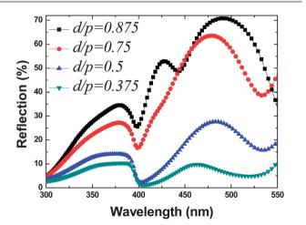
**Fig. 3** Calculated reflection of nanorod arrays with constant periodicity p = 400 nm and varying inter-rod gaps and diameters corresponding to different d/p values ranging from 0.375 to 0.875.
