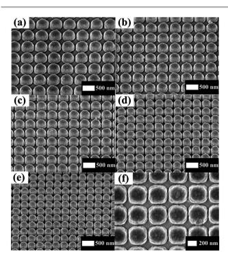
**Fig. 4** SEM images showing oblique views of dense nanorod arrays with different periodicities from (a) 540 nm to (e) 320 nm with a step size of 55 nm. (f) Magnified top view of (d) with p = 375 nm and d = 350 nm.
