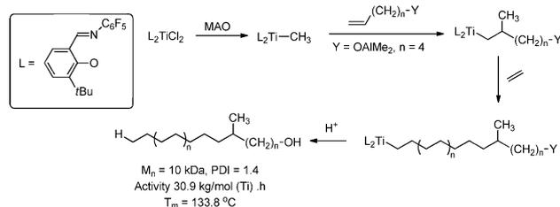
**Scheme 27** Introduction of functional groups during the initiation of polyethylene growth using a titanium catalyst bearing phenoxyimine (FI) ligands.
