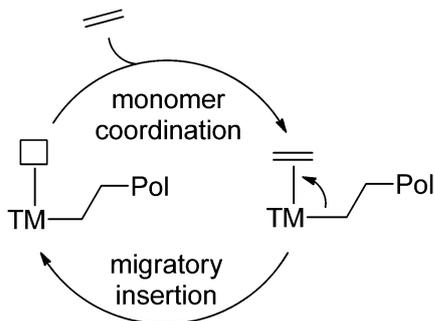
**Scheme 12** Schematic representation of TM-catalysed coordination/insertion polymerisation.
