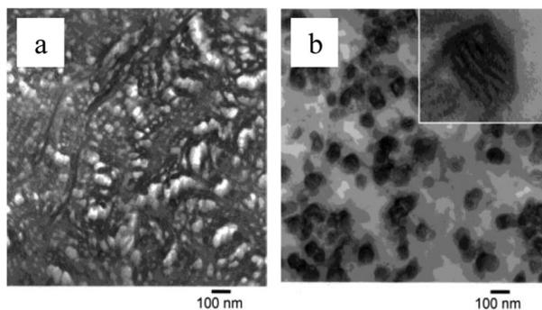
**Fig. 3** TEM pictures of polypropene-polymethylmethacrylate block-copolymers (PP-*b*-PMMA) showing phase separation at the microscopic level, with different morphologies for a PMMA content of 60% (a) and 75% (b).<sup>181</sup> (Reproduced with permission; Copyright 2003 Wiley)
