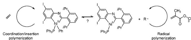
**Scheme 41** Reversible shuttling process between a Ni<sup>II</sup> species responsible for coordination/insertion polymerisation of ethene and a Ni<sup>I</sup> species active in controlled radical polymerisation of acrylates. Multiple shuttling cycles result in the formation of ethene-acrylate multiblock copolymers.
