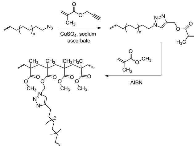
**Scheme 47** PE macro-initiator prepared *via* catalytic chain-shuttling (see also Scheme 31) and subsequent ‘click’ reaction with propargyl methacrylate. The obtained macro-monomer was used in a radical copolymerisation with methyl methacrylate to obtain PMMA-*g*-PE copolymers.
