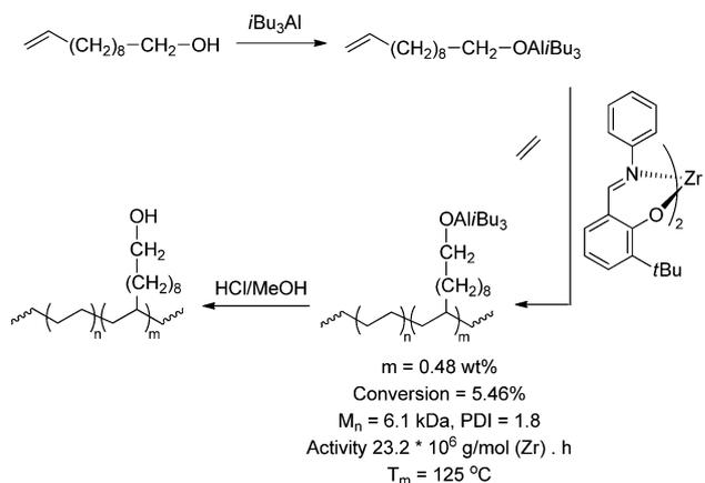
**Scheme 14** Synthesis of polyethene containing alcohol functionalities *via* direct copolymerisation with aluminium-protected OH-functionalised monomers.
