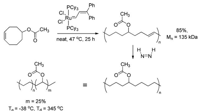
**Scheme 3** Synthesis of functionalised polymers resembling copolymers of ethene and vinyl acetate via ROMP followed by hydrogenation.
