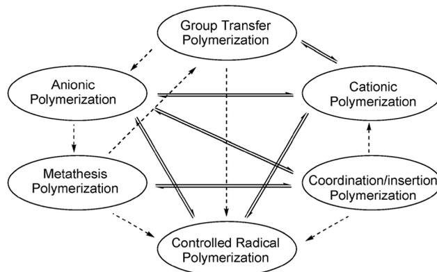
**Fig. 4** Mechanistic transformations in living/controlled polymerisation aimed at the synthesis of block copolymers. Solid lines indicate pathways suitable for the synthesis of functional polyolefins, while pathways indicated with dashed lines are not.
