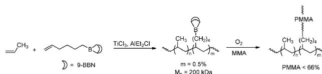
**Scheme 44** Synthesis of PP-*g*-PMMA copolymers *via* ETM catalysed coordination/insertion polymerisation followed by peroxyborane-initiated radical polymerisation. The borane initiation sites were incorporated in the polymer backbone *via* direct copolymerisation of borane-functionalised monomers with propene.
