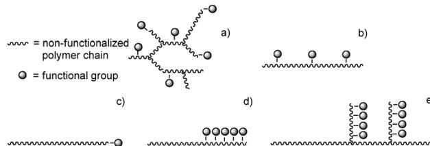
Fig. 2 Functionalised polyolefins divided into 4 classes based on structural differences: randomly functionalised copolymers (a and b), chain-end functionalised polymers (c), block copolymers (d), and graft copolymers (e).
