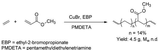
**Scheme 10** Ethene-acrylate copolymers prepared *via* ATRP.
