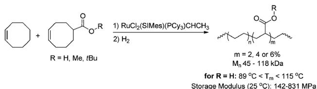
**Scheme 5** Synthesis of analogues of ethene-acrylate copolymers obtained by ROMP copolymerisation of functionalised and non-functionalised cyclooctenes containing theoretically 2, 4 or 6% incorporation of polar vinyl monomers.
