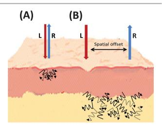
**Fig. 4** Simplified graphical representation of (A) spontaneous Raman compared to (B) spatially offset Raman scattering, illustrating the spatial offset and deeper subsurface probing in skin tissue. L = laser light, R = Raman light.
