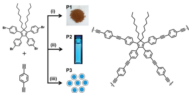
Scheme 1 Fabrication of porous organic polymers involving TBDC (tetakis-(4-bromophenyl)-5,5-dioctylcyclopentadiene) and DEB (diethynylbenzene) in the form of powder ( P1 ), soluble in organic solvents ( P2 ) and aqueous dispersion of nanoparticles ( P3 ). Fabrication conditions: (i) [Pd(PPh 3 ) 4 ], CuI, diisopropylamine, toluene, 80 °C, 48 h, (ii) [Pd(PPh 3 ) 2 Cl 2 ], CuI, diisopropylamine, toluene, 80 °C, 12 h and (iii) [Pd(PPh 3 ) 4 ], CuI, SDS, water, diisopropylamine, toluene, 50 °C, 48 h.
