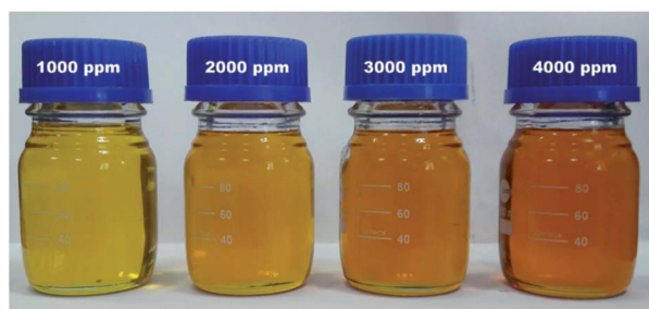
Fig. 6 Solubility of synthesized PzP(-NHP)_6 in polyol in different concentrations.
