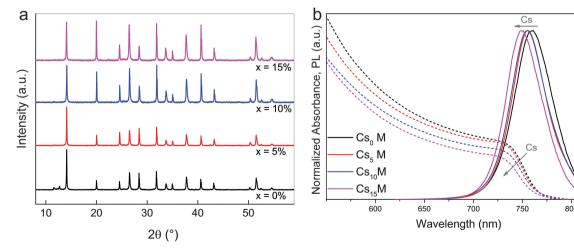
Fig. 1 XRD and optical characterisation of Cs<sub>v</sub>M compounds. (a) XRD spectra of perovskite upon addition of Cs investigating the series  $Cs_x(MA_{0.17}FA_{0.83})_{(1-x)}Pb(I_{0.83}Br_{0.17})_3$ , abbreviated as  $Cs_xM$  where M stands for "mixed perovskite".  $Cs_xM$  with x = 0, 5, 10, 15%. (b) The corresponding (dashed lines) and photoluminescence (PL) spectra (solid lines).
