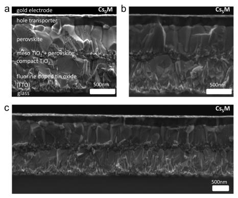
Fig. 3 Cross-sectional scanning electron microscopy (SEM) images of (a) Cs₀M (b) Cs₅M and (c) low magnification Cs₅M devices.
