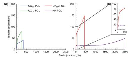
Fig. 3 Tensile test of the PCL film mechanical properties. (a) Representative stress-strain curves of  $UX_{SC}$ -PCL,  $UX_{CS}$ -PCL,  $UX_{CS}$ -PCL and HP-PCL. (b) The enlarged portion of UX<sub>HP</sub>-PCL and HP-PCL stress-strain curves.
