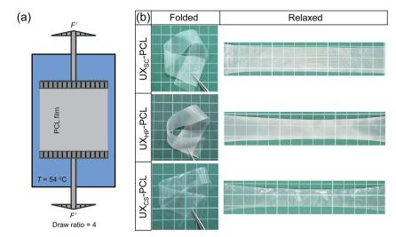
Fig. 1 (a) Schematic illustration of the fabrication set-up for uniaxial thermal stretching of PCL films (T = 54 °C; draw ratio = 4). (b) Uniaxially stretched flexible PCL films experiencing the bending and folding, and recovering to their original status. UX<sub>SC</sub>-PCL, UX<sub>HP</sub>-PCL and UX<sub>CS</sub>-PCL representing the stretched films with a pre-fabrication of solvent cast (SC), heat press (HP) and cast stretch (CS), respectively.
