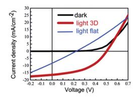
Fig. 10 (a) Schematic picture of a nanocomposite 3D solar cell, and (b) J-V characteristics of the 3D solar cell based on a  $TiO_2/In_2S_3/CuInS_2$  nanocomposite. Reprinted with permission from ref. 80, Copyright 2005, American Chemical Society.
