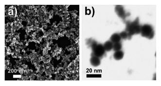
Fig. 13 Electron microscopy of citrate-capped Cu<sub>11</sub>In<sub>9</sub> nanoparticles: (a) SEM overview image, and (b) detailed bright-field STEM image. Reprinted with permission from ref. 86, Copyright 2011 American Chemical Society.
