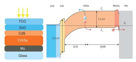
Fig. 2 Left – a schematic layer structure of a classical CIGSe solar cell. Right – a schematic band profile of a typical CIGSe solar cell under zerobias voltage condition. The image of the band profile is reprinted with permission from ref. 12, Copyright 2011, Nature Publishing Group.
