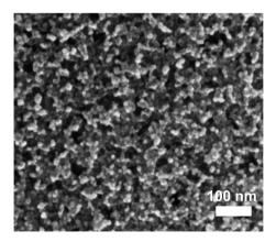
Fig. 8 (a) SEM top view image of a CuInS<sub>2</sub> NC film formed by an in situ deposition of precursor solution, sintered at a temperature of 270 °C. Reproduced with permission from ref. 28, Copyright 2013, Wiley VCH.
