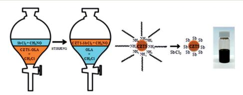
Fig. 19 Schematized view of the procedure representing the ligand-exchange of the long-chain OLA ligand with an inorganic salt SbCl<sub>3</sub>. Reprinted with permission from ref. 157, Copyright 2013 American Chemical Society.
