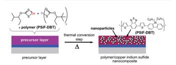
Fig. 16 Schematic representation of the polymer/CIS nanocomposite formation. Reprinted with permission from ref. 139, Copyright 2011, Wiley VCH.
