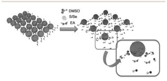
Fig. 5 Schematic representation of the dissolution mechanism for Cu-In hydrazinium in a solvent mixture of EA and DMSO. Reprinted with permission from ref. 63, Copyright 2012, Wiley VCH.
