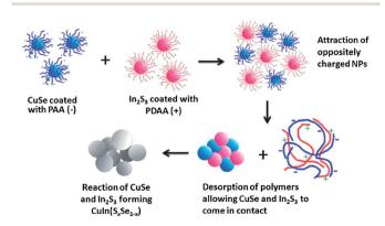
Fig. 14 A schematic diagram representing the formation of CulnS<sub>x</sub>Se<sub>1-x</sub> nanoparticles through electrostatically induced coalescence and sintering of binary CuSe and In<sub>2</sub>Se<sub>3</sub> nanoparticles. Reprinted with permission from ref. 120, Copyright 2013, The Royal Society of Chemistry.
