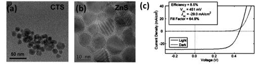
Fig. 18 TEM pictures of (a) CTS and (b) ZnS nanoparticles and the corresponding (c) J-V curves of CZTSSe devices. Reprinted with permission from ref. 151, Copyright 2012 American Chemical Society.
