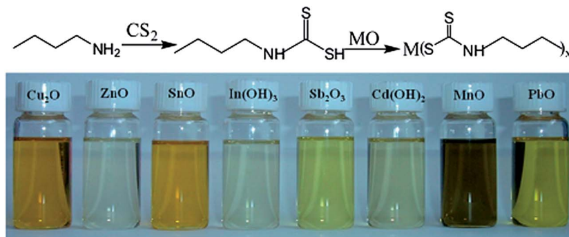
Fig. 9 (Top) Reaction mechanism of a metal oxide with butyldithiocarbamic acid. (Bottom) Digital photograph of various metal oxides dissolved in chloroform with the aid of butylamine and carbon disulfide ( \sim 0.35 M metal acid concentration). Reprinted with permission from ref. 73, Copyright 2012 American Chemical Society.
