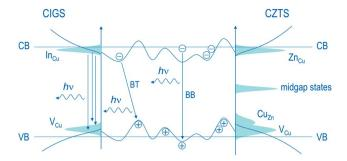
Schematics of the band diagram for Cu-poor CIGSe and Cupoor, Zn-rich CZTS, which represent the dominance of the band-tail (BT) and band-to-band (BB) transitions between delocalized donor and acceptor states. The energetic bands show potential fluctuations due to the local deviations in the distribution of donor and acceptor states. Reprinted with permission from ref. 22, Copyright 2011, American Physical Society.
