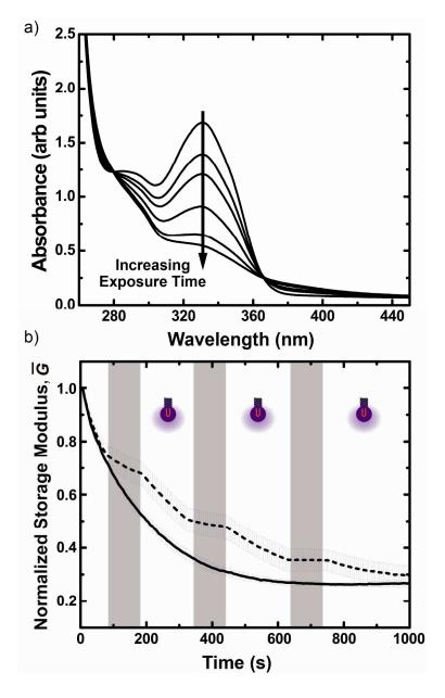
**Figure 2.** a) UV-vis spectra of poly(MAA-*co*-BHCMM)-PEG-poly(MAA-*co*-BHCMM) in DMSO solution before and after UV exposure. Uncaging is evident by the decrease of absorbance peak at 330 nm. b) The temporal evolution of normalized storage modulus G' is plotted for continuous (solid line) and intermittent (dashed line) exposure to UV irradiation. White (grey) vertical bars correspond to the presence (absence) of UV illumination.
