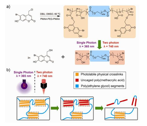
**Figure 1.** a) Synthesis and photodeprotection schemes for poly(MAA-*co*-BHCMM)-PEG-poly(MAA-*co*-BHCMM) ABA triblock copolymers is shown. Light-induced uncaging of PBHCMM segments yields water soluble PMAA-PEG-PMAA ABA triblock copolymers. b) A schematic illustration that describes the proposed mechanism of light-induced phase inversion and disintegration of physically crosslinked hydrogels.
