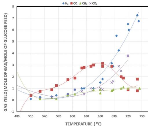
Fig. 11 Diagram showing the variation in product distribution vs. reactor temperature in SCWG.<sup>121</sup>
