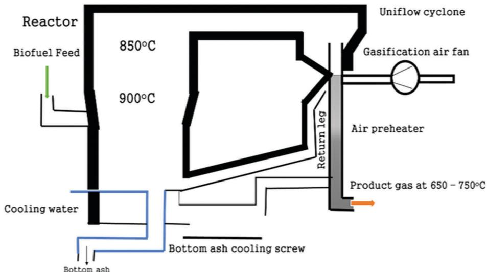
Fig. 2 Schematic diagram of a conventional fluidized bed gasifier (circulating).<sup>28</sup>
