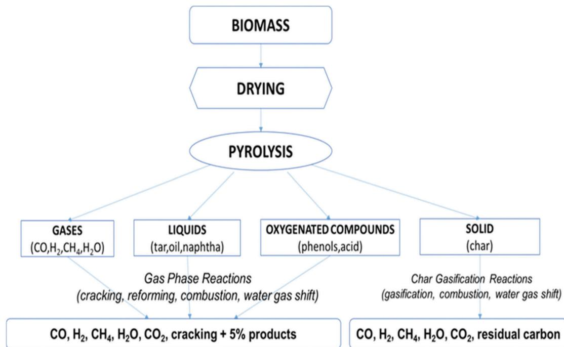
Fig. 4 Gasification routes.<sup>31</sup>
