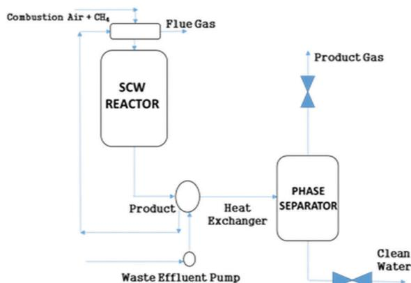
Fig. 10 Simplified schematic of SCWG.<sup>120</sup>
