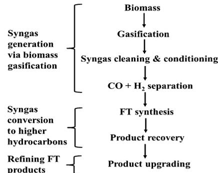
Fig. 15 Flow chart depicting FT-fuel synthesis from biomass.
