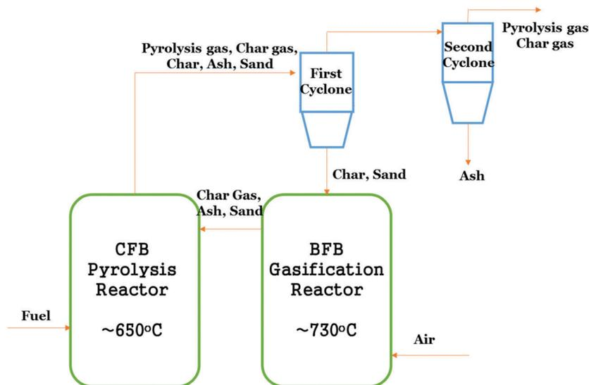
Fig. 7 Simple schematic diagram of LT-CFB gasifier.<sup>3</sup>
