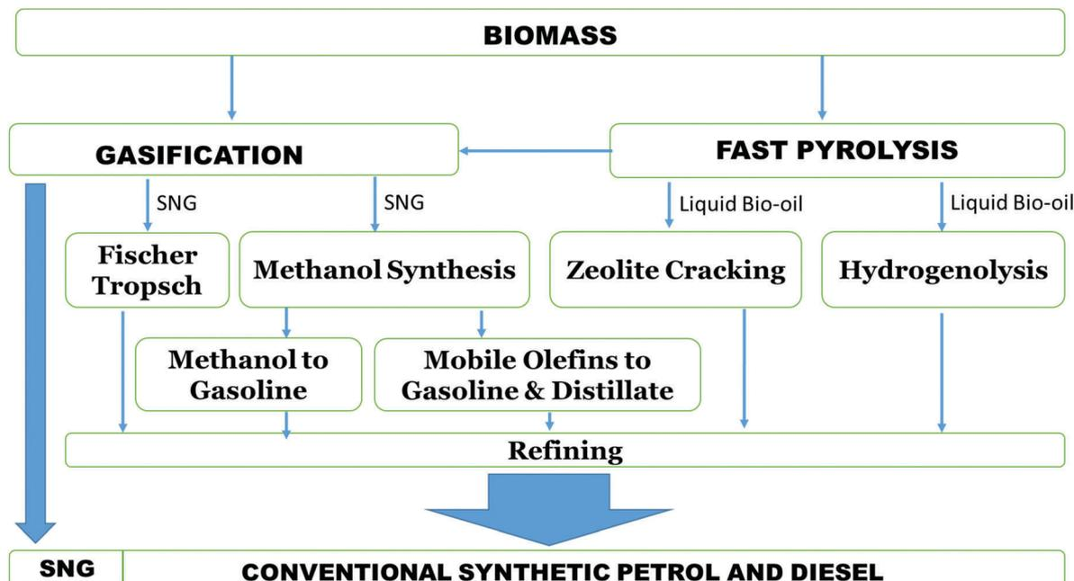
Fig. 13 Biomass gasification and pyrolysis routes to synthetic biofuels.<sup>208</sup>
