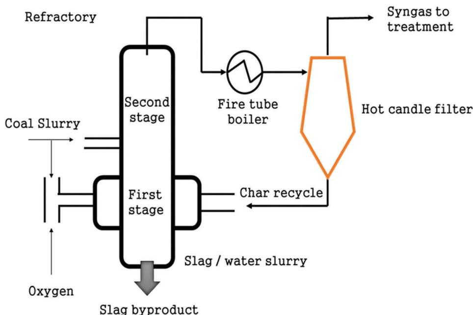
Fig. 3 Schematic diagram of an entrained flow gasifier (side-fed).<sup>28</sup>
