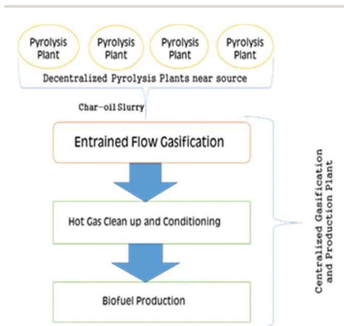
Fig. 8 Simplified scheme of the Bioliq concept.
