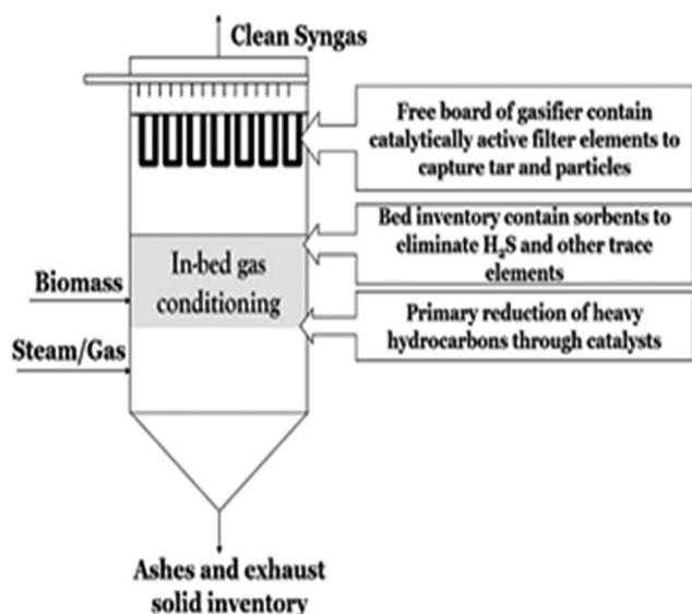
Fig. 5 Schematic of unique combination of gasification with *in situ* gas cleaning and conditioning.<sup>3</sup>
