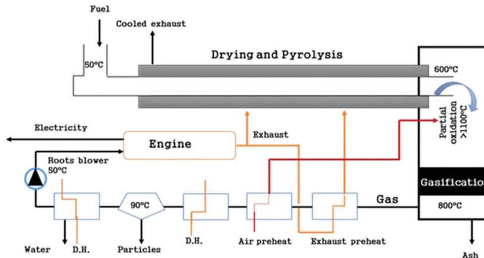
Fig. 6 Schematic diagram of Viking gasifier.<sup>84</sup>
