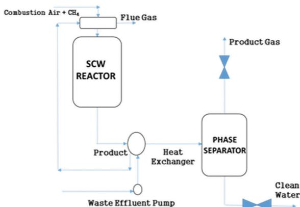
Fig. 10 Simplified schematic of SCWG.<sup>120</sup>
