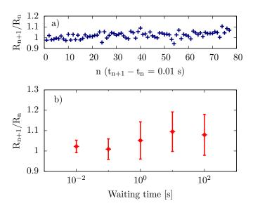
**Fig. 5** Analysis of the system stability during the waiting time  $\Delta t$  between two subsequent I-V measurements. a) The ratio of the  $(n+1)^{th}$  and  $n^{th}$  resistances  $R_{n+1}/R_n$  at  $V_{drive} = 0$  V applied during  $\Delta t = 0.01$  s. b) The average and standard deviation of  $R_{n+1}/R_n$  as a function of  $\Delta t$ .
