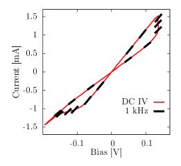
**Fig. 4** I-V trace recorded at a slow bias signal of f = 1 Hz (red). The results of a simultaneous lock-in measurement performed at an AC modulation of f = 1 kHz along the DC curve are represented by the black dashes.
