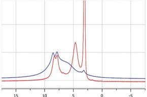
Fig. 2 (red) <sup>1</sup>H-NMR of UiO-67 immediately after vacuum filtration. (blue) <sup>1</sup>H-NMR of UiO-67 6 days after vacuum filtration. The corresponding <sup>13</sup>C-NMRs can be seen in Fig. S2 (ESI†).
