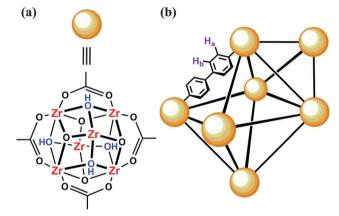
Fig. 1 (a)  $Zr_6O_4(OH)_4$  cluster showing 4 of the 12  $\mu$ -BPDC units. (b) Schematic drawing of UiO-67 illustrating how the BPDC units link Zr<sub>6</sub>O<sub>4</sub>(OH)<sub>4</sub> clusters to one another to form both octahedral- and tetrahedral-shaped pores.
