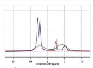
Fig. 4 (red) <sup>1</sup>H-NMR of UiO-67 immediately after thermal activation from acetone. (blue) <sup>1</sup>H-NMR of UiO-67 4 days after thermal activation. (green)  $^{1}$ H-NMR of UiO-67  $^{1}$  month after thermal activation. The corresponding <sup>13</sup>C-NMRs can be seen in Fig. S4 (ESI†).
