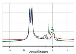
Fig. 3 (red) <sup>1</sup>H-NMR of UiO-67 immediately after thermal activation from methanol. (blue) <sup>1</sup>H-NMR of UiO-67 4 days after thermal activation. (green)  $^{1}$ H-NMR of UiO-67  $^{1}$  month after thermal activation. The corresponding <sup>13</sup>C-NMRs can be seen in Fig. S3 (ESI†).
